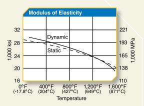
Data are typical and should not be construed as maximum or minimum values for specification or for final design. Data on any particular piece of material may vary from those herein. Copyright © ATI Allvac 2010. ATI 718-OP® and Allvac® are registered trademarks of ATI Properties, Inc.
