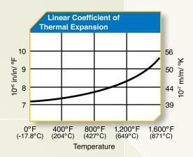
Data are typical and should not be construed as maximum or minimum values for specification or for final design. Data on any particular piece of material may vary from those herein. Copyright © ATI Allvac 2010. ATI 718-OP® and Allvac® are registered trademarks of ATI Properties, Inc.
