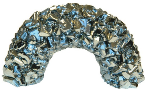
Figure 1. Hafnium Crystal Bar from the van Arkel / deBoer iodide process
