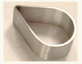
Testing at 1200°F resulted in minimal attack for both the ATI 332Mo<sup>™</sup> and 625 alloy samples. The weight gain was small and positive, indicating that the corrosion products were adherent and relatively protective. The Type 316Ti sample exhibited significant attack manifested as a net weight loss, indicating that the corrosion products were loss and non-protective.
