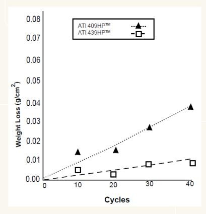
ATI 439™ alloy (UNS S43035) with its higher chromium content is shown to offer significantly improved corrosion resistance (lower weight loss) than the ATI 409 alloy. Published information emphasizes that chlorides, which may be present on startup of new automobiles or new catalytic convertors due to carryover from catalytic converter manufacture, makes the initial condensate more aggressive than would be expected at normal automotive operating conditions.
