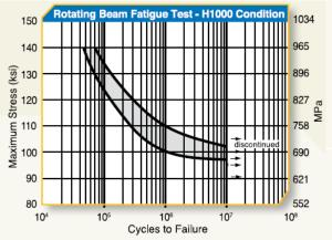
H1000 Solution Heat Treated and Aged Condition Rotating Beam Fatigue Room temperature R = -1
