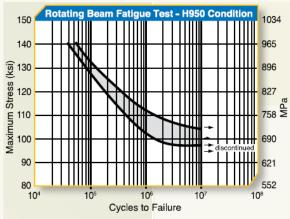
H950 Solution Heat Treated and Aged Condition Rotating Beam Fatigue Room temperature
