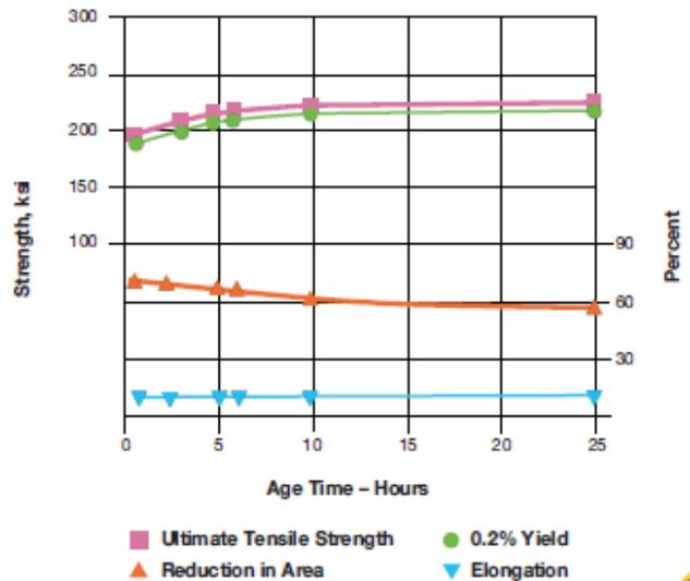
All specimens solution annealed for one hour at 1,500°F, air cooled and aged at 900°F for the times indicated.
