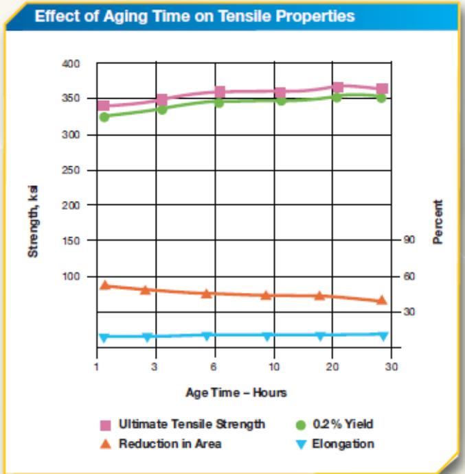
All specimens solution annealed for one hour at 1,500°F, air cooled and aged at 900°F for the times indicated.
