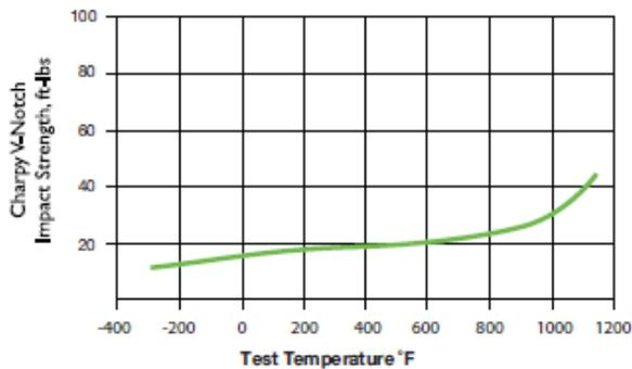
All specimens solution annealed for one hour at 1,500°F, air cooled and aged at 900°F for the times indicated.
