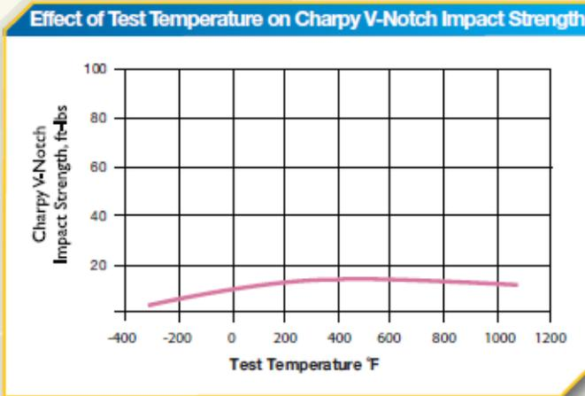
All specimens solution annealed for one hour at 1,500°F, air cooled and aged at 900°F for the times indicated.
