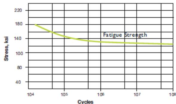
All specimens solution annealed for one hour at 1,500°F, air cooled and aged at 900°F for the times indicated.
