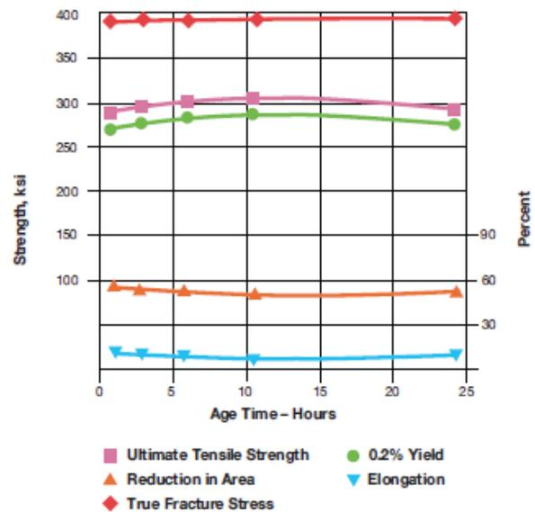
All specimens solution annealed for one hour at 1,500°F, air cooled and aged at 900°F for the times indicated.
