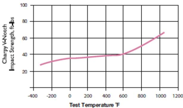
All samples solution annealed for one hour at 1,500°F, air cooled and aged at 900°F for three hours.
