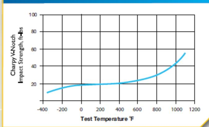
All samples solution annealed for one hour at 1,500°F, air cooled and aged at 900°F for three hours.
