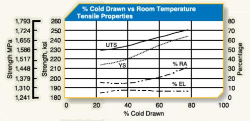
Note: Starting with .373" diameter rod, solution annealed, drawn, aged at 900° F for 6 hours, AC.
