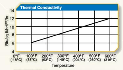
Note: Conductivity for as-rolled and heat treated + aged samples is equivalent.
