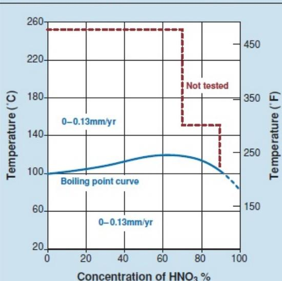
The corrosion resistance of titanium alloys can depend on the presence of multivalent impurities for passivation of the surface to reduce corrosion. Zirconium does not require the presence of multivalent ions for its corrosion resistance.
