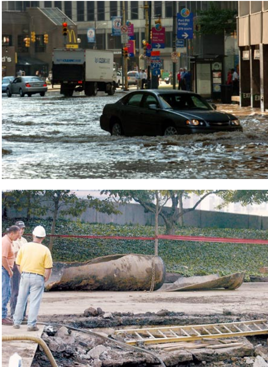
Figure 2: The top image shows the flooding in downtown Pittsburgh that resulted from the fractured cast iron pipe shown in the lower image 7 .
