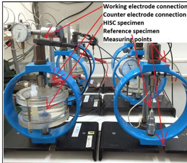
**Figure 3. Cortest ring setup for Method I testing showing the configuration of the pre-charged sample in the test environment.**
