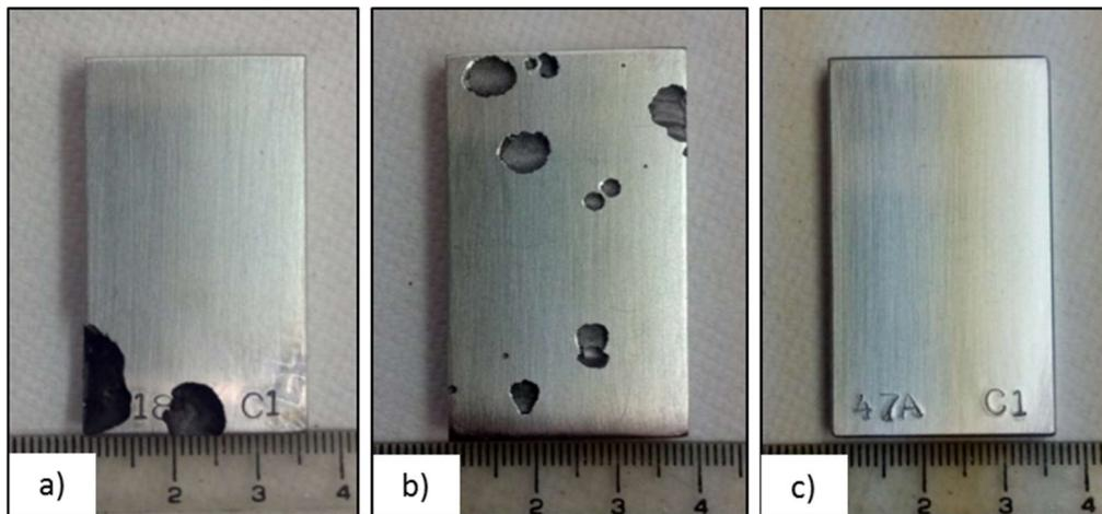
**Fig 2: Comparison of common nickel alloys to ASTM G48C pitting corrosion test at 50 °C**
