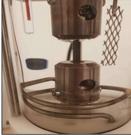
**Figure 4: Shows a notched SSRT hydrogen charged sample. The Ag/AgCl reference electrode is seen in the upper left, and the Pt-counter electrode on the right.**
