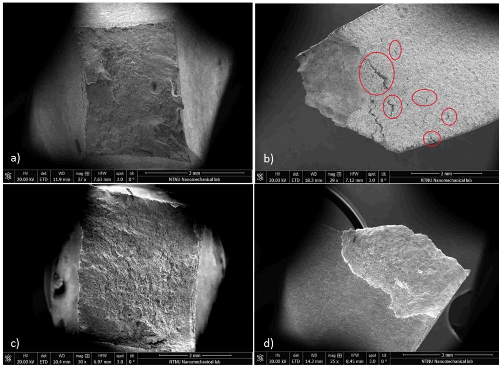
**Fig 6: ISL fracture surfaces for rectangular test specimens of N08830 alloy. Top a and b) fracture surface and secondary cracks of the smooth sample. Bottom c and d) fracture surface of the notched sample showing mostly ductile fracture with no secondary cracking.**
