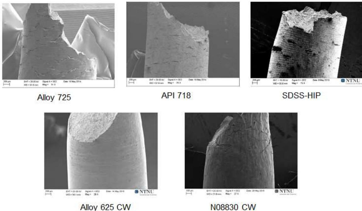
**Fig 5: ISL round-smooth fracture samples comparing alloys' secondary cracking.**
