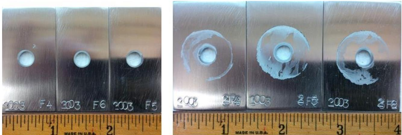
Figure 5. ATI 2003® alloy after crevice corrosion testing in acidified ferric chloride showing the difference in attack of the MCA (left) and the single crevice assembly (right) at 15 °C.
