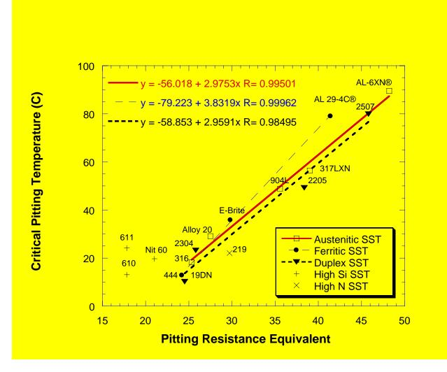
Figure 10: Critical Pitting Temperature as a function of Pitting Resistance Equivalent (PRE) number for austenitic, duplex, and ferritic stainless alloys.<sup>(15)</sup>
