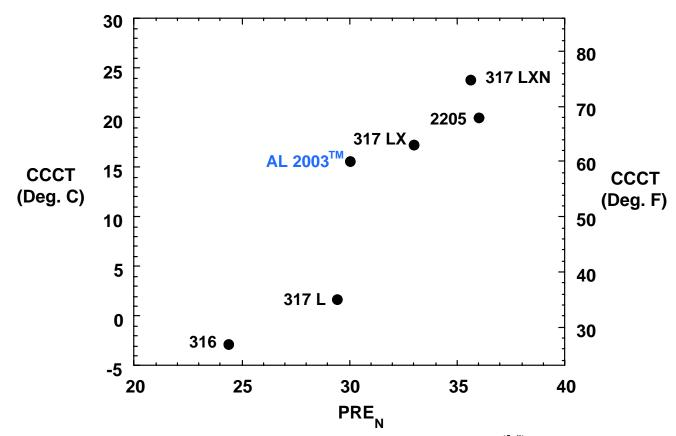
Figure 7: Critical Crevice Corrosion Temperature per ASTM G48C vs.  $\text{PRE}_{N}^{\ (5,\ 8)}$
