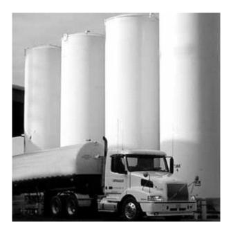
Figure 5: Cryogenic Vessels for liquidified gases of UNS S20153 alloy
