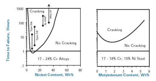
Figure 9: Effect of nickel (left) and molybdenum (right) on SCC resistance in boiling magnesium chloride solutions <sup>(13)</sup>
